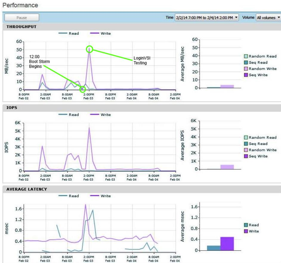
Figure 2 - Nimble CS220G-X4 metrics shown with boot storm and LoginVSI test
